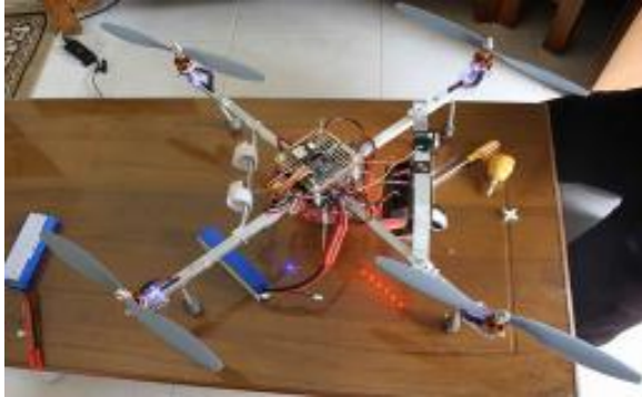
Gambar 3. Perakitan wahana Quadcopter
